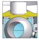
**1. Low sump area** seamless connection to vessel inner wall.
