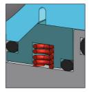
2. Spring loaded sealing system
